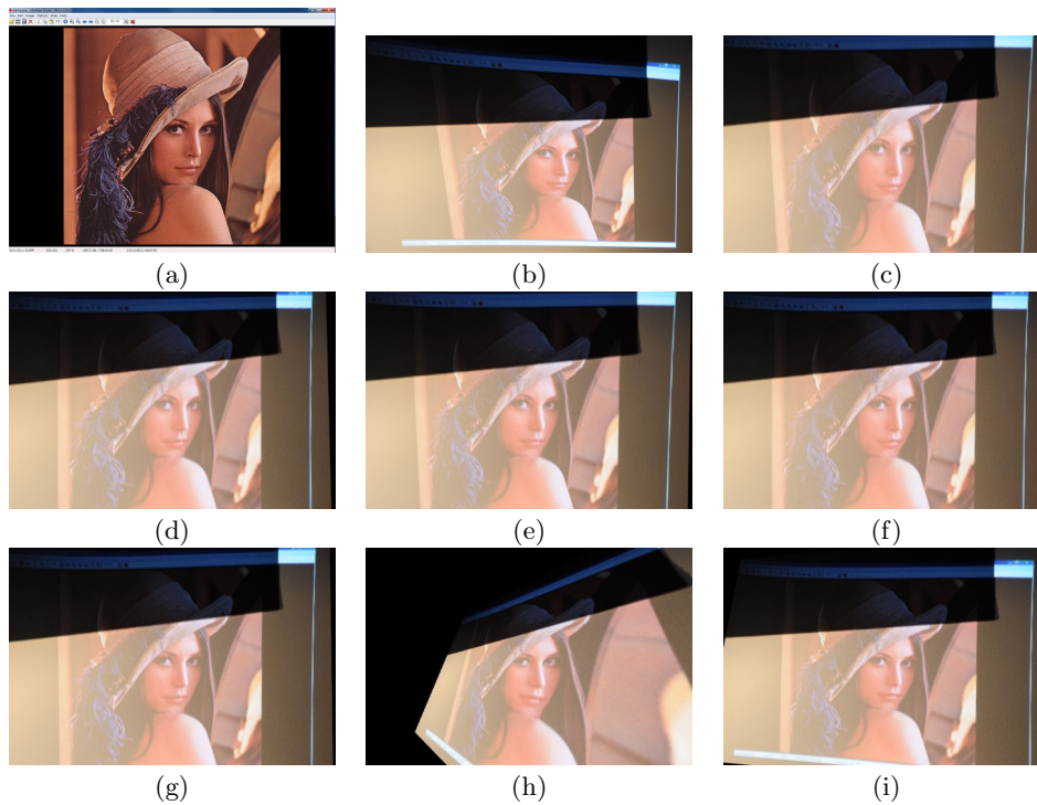
Figure 4: Real homography transform estimation experiments. (a) Projected image; (b) Captured image; The following images compensated by : (c) SURF; (d) SURF with LHE; (e) RGB SURF; (f) RGB SURF with LHE; (g) SURF with GHE; (h) HSV SURF; (i) Opponent SURF.
