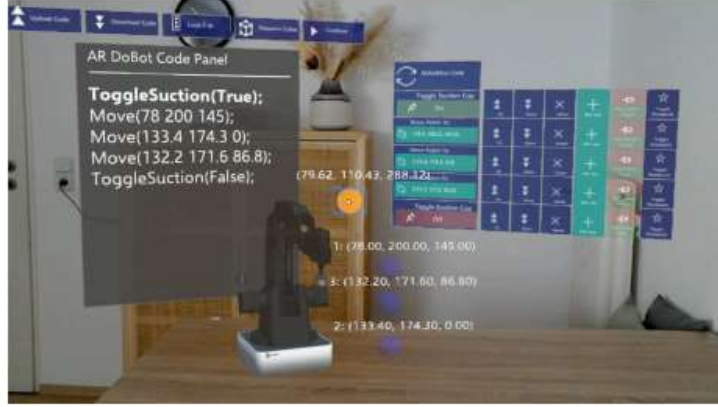
Fig. 6: Robot Code, Robot Model in an AR application and block-based DSL Code (f.l.t.r.)
