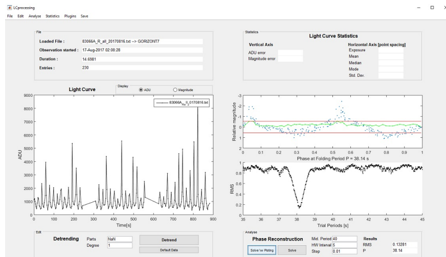
Fig. 5: Main GUI components of the FMPI's matlab script LCProcessing.m used for the time series analysis and phase diagram construction.
