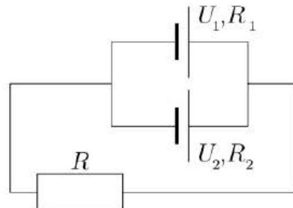
a.  $I = \frac{U_1 R_2 + U_2 R_1}{R_1 R_2 + R(R_1 + R_2)}$
