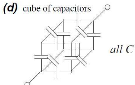
Use symmetries of the configurations to calculate their total capacitances.
