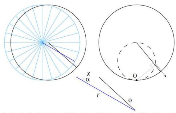
As the wheel rolls to the right, it rotates clockwise. A spoke shifts to the right by distance x and rotates by angle  $\phi$  that are related
