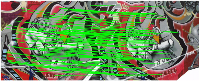
Figure 2: An example of matching pairs of keypoints between two images using our proposed Color-BRIEF descriptor.
