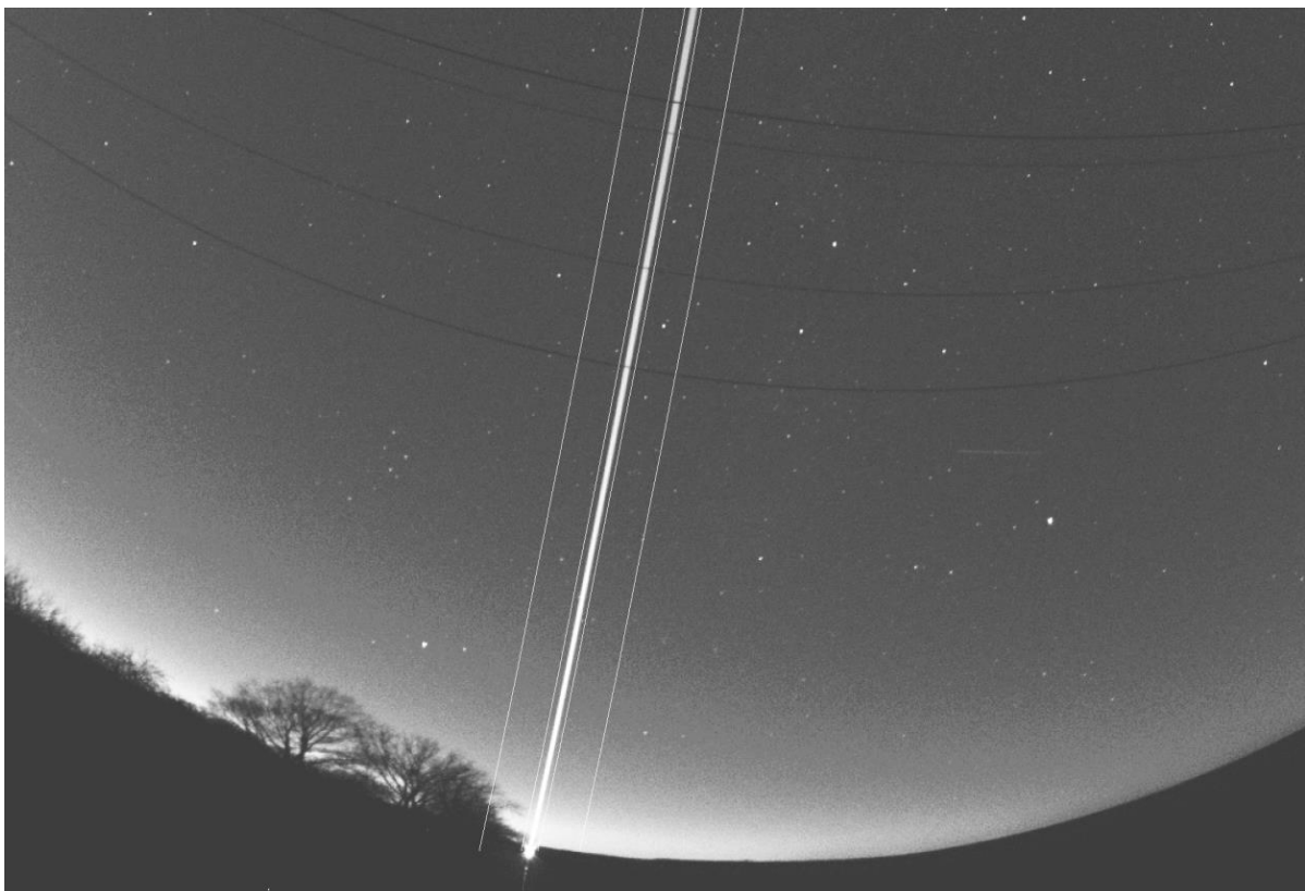
Fig. 11. A cut from 'linearlyscaledG.pgm' file. The laser beam is located in the central band. Both side-bands are also shown. A few power lines crosses the image of the laser beam. No background image subtraction was applied.
